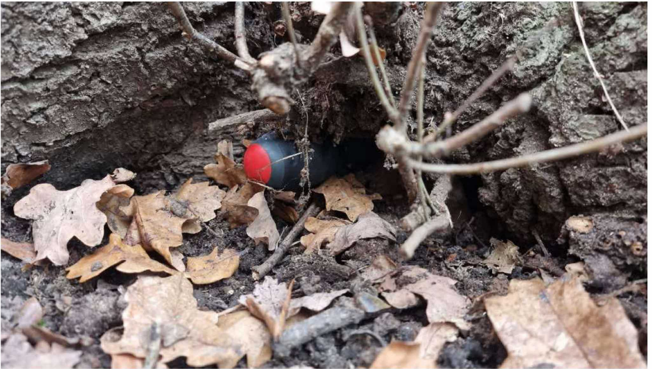
T1 oak photo 1 - Screwdriver inserted into the decay at the base between the buttress roots on the south side
